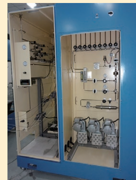
Gas flow rate control equipment
