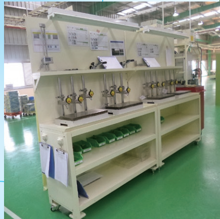
Dolly for holding measuring device
